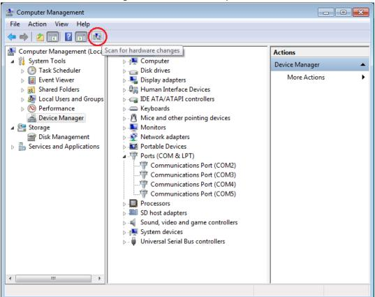
3. The COM ports should appear as COM1 and COM6 when installed
