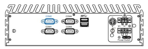
Serial port COM2 can be configured for RS-232, RS-422, or RS-485 with auto flow control. The default setting for COM2 is RS-232. Configuration of COM2 can be done in the BIOS settings.
