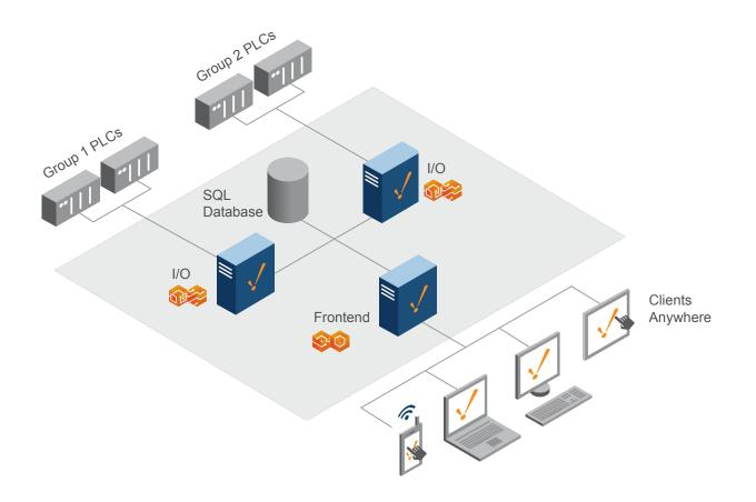
With this architecture, you have two Ignition servers communicating to different sets of PLCs, allowing for communication to a larger set of devices and tags. For example, it is possible to handle approximately 250,000 tags from 200 devices. You can easily add additional I/O servers as necessary.
