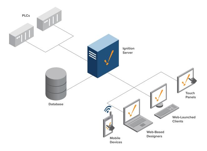
Ignition's most common architecture consists of a single on-premise Ignition server connected to a SQL database, PLCs, and clients. In this case, all functionality is configured on the same Ignition server. Ignition's licensing is unlimited. However, Ignition is limited by the size of the hardware. With larger hardware, Ignition can handle more device connections, tags, and clients.
