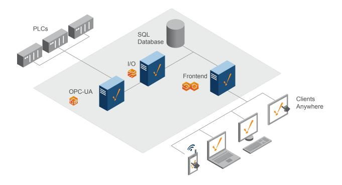
With this architecture, a dedicated OPC-UA server that handles all of the PLC communication was introduced. Essentially, you are breaking apart OPC-UA from a single server. This architecture lets one handle a larger set of devices. The I/O server simply handles the tag value changes. You can easily handle a larger set of tags, in regards to history and alarming, with additional OPC-UA servers for different sets of PLCs.
