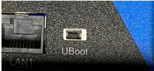
Press and hold this button while powering on the panel.
